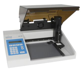
Spray-on technique: high accuracy and perfectly reproductible sample deposits Dual syringe system: dosing and filling syringe Low sample requirement Application of dots or lines Protective cover prevents external contamination Circuit rinsing before each application Stand-alone or PC-controlled Easy-to-use software, transferring data to Densitometer CD60 Holding up to 10 methods Volume spotted on the HPTLC plate: from 0.1µl to 1 ml Can be easily upgraded to fully automatic
