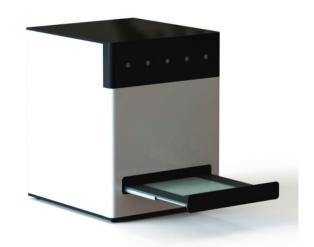
The ProViDoc DD80 is a high-performance documentation system with brilliant recording quality. The workstation consists of a dark hood with different light sources, a camera for taking high-resolution images, a documentation top for guaranteeing the optimal distance between camera and sample as well as a software for controlling the system and saving the recorded images.
